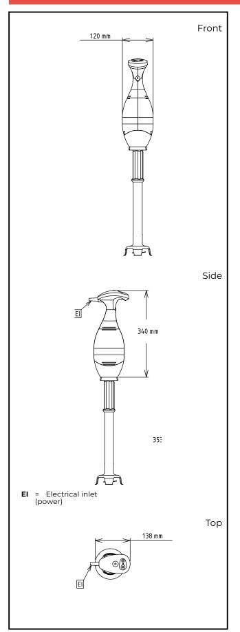
Electric Supply voltage: 220-240 V/1 ph/50/60 Hz **Electrical power max.:** 0.75 kW 0.75 kW **Total Watts:** Capacity: Performance (up to): **Capacity:** 290 litres Key Information: External dimensions, Width: 138 mm External dimensions, 120 mm Depth: External dimensions, Height: 965 mm 6 kg **Shipping weight:** Net weight (kg): 3.7 **Cold water paste: Egg whites:**
